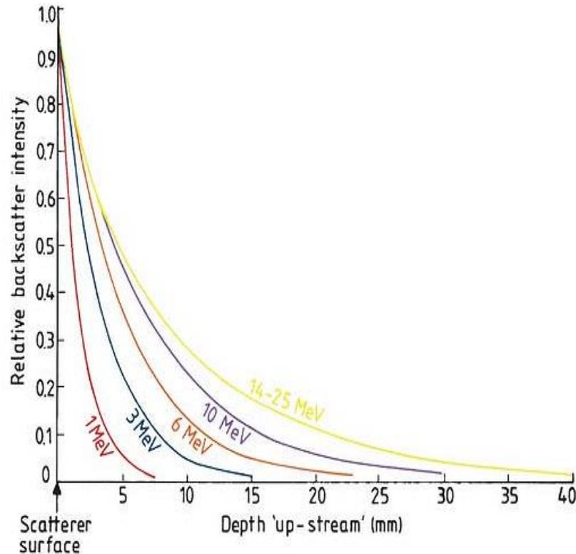
To dissipate the effect of electron backscatter, a suitable thickness of low Z absorber may be placed between the lead shield and the preceding tissue surface
